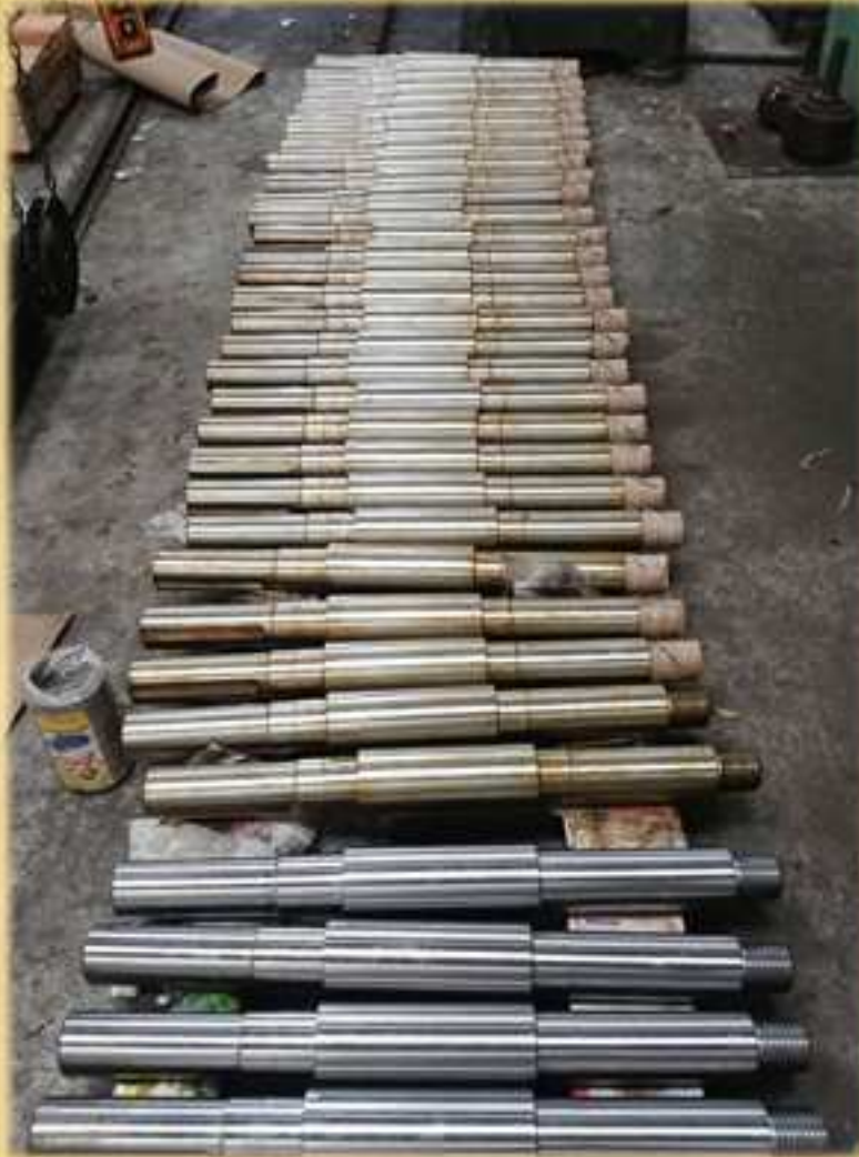
Horizontal Slurry Pump Shafts ( Moc: EN8, SS316, EN19, EN24, SS304 etc)
