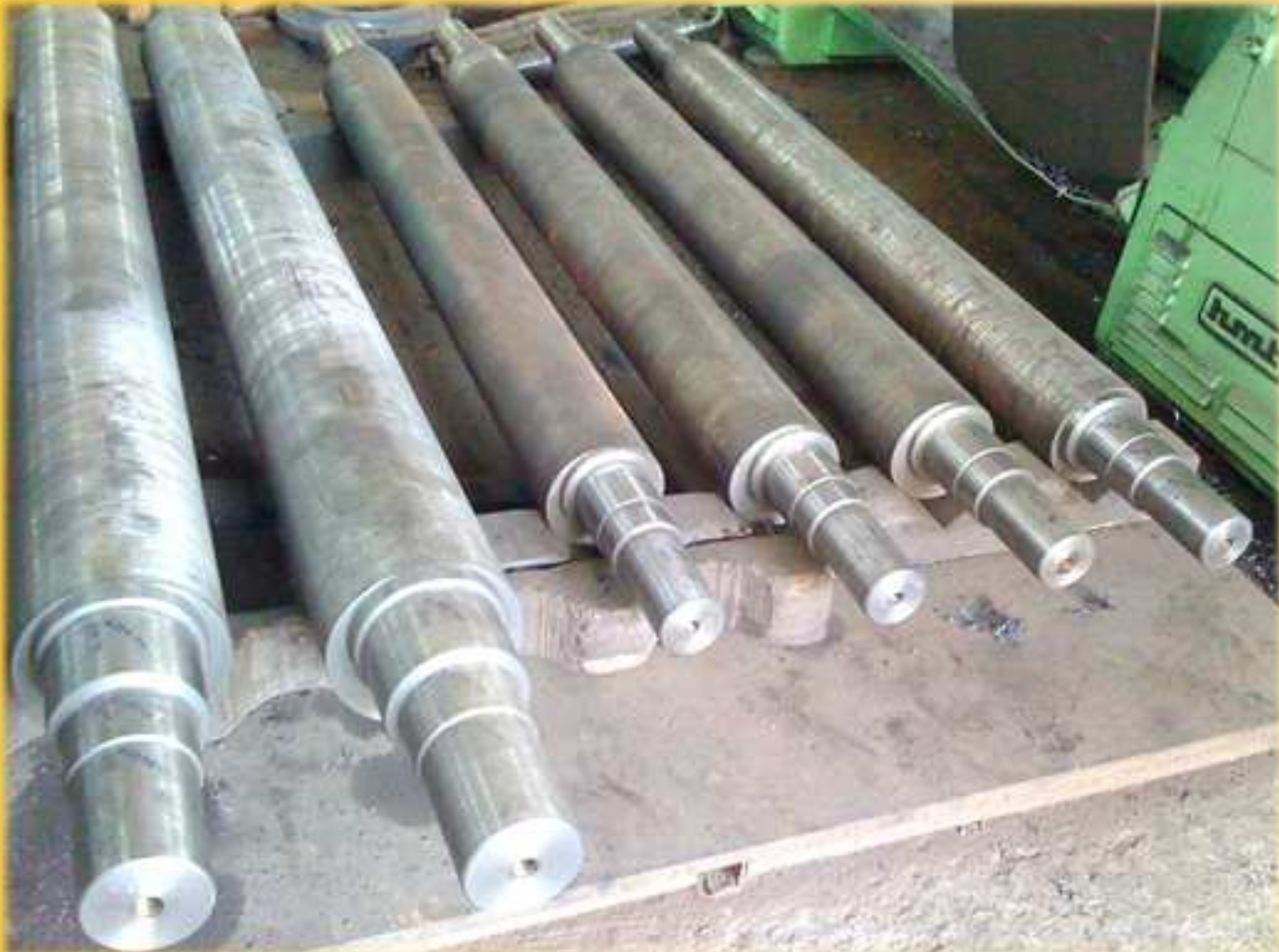
Eccentric Shafts for Multiple Deck Vibrating Mining Screens (Eccentricity is up to 35mm)
