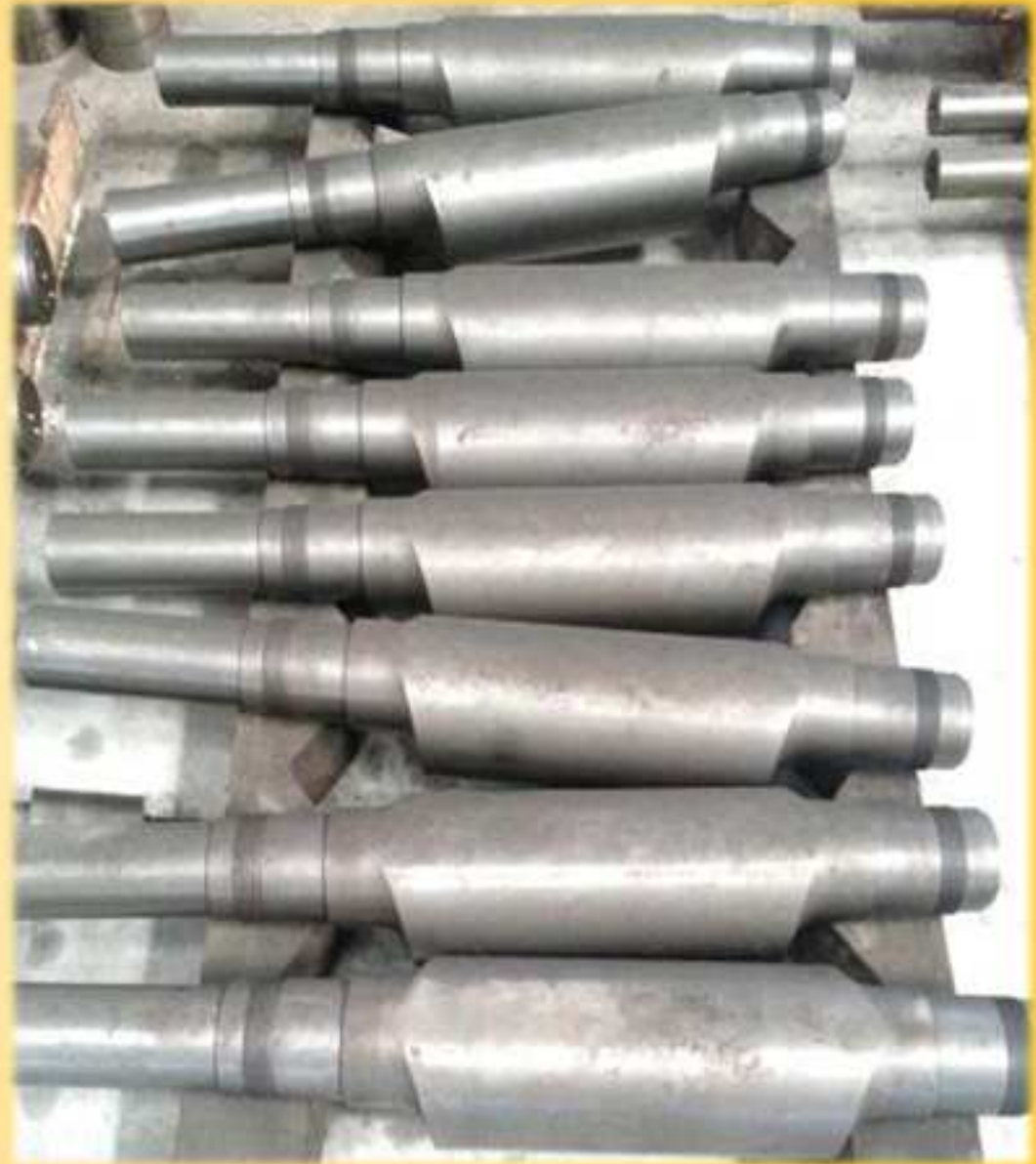
Main Eccentric Shafts of Jaw Crushers (Eccentricity is up to 40mm)
