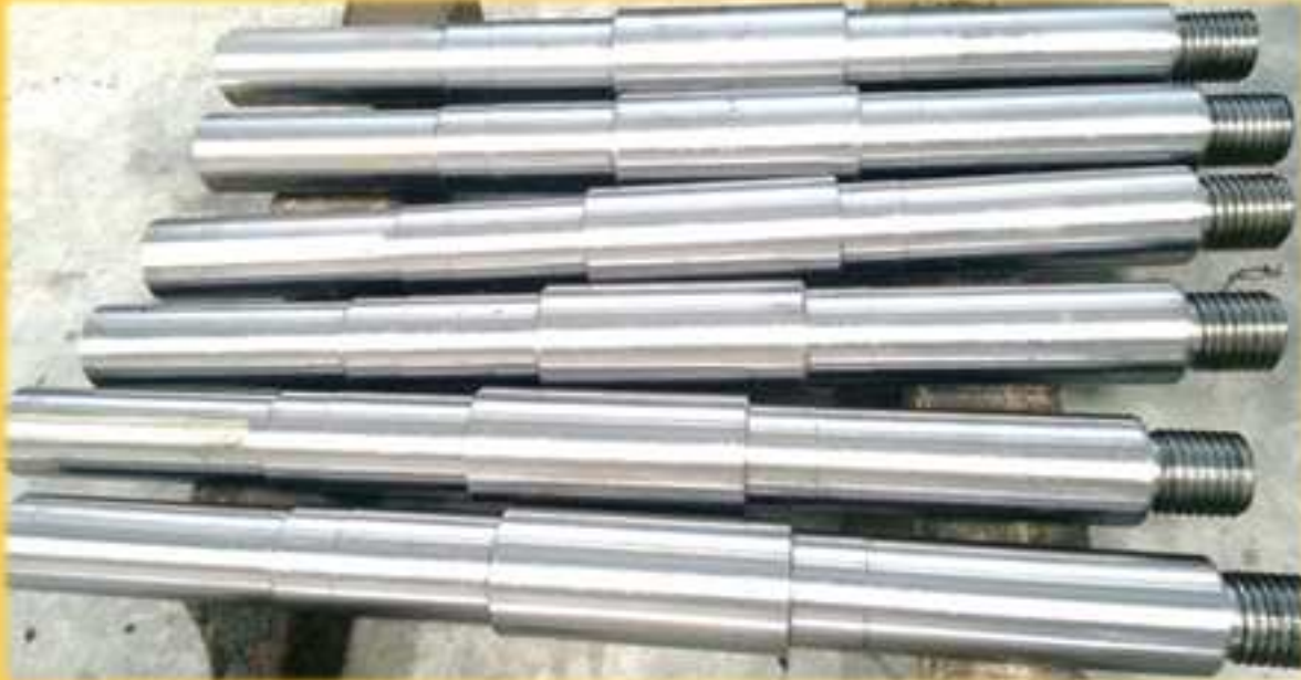
Slurry Pump Shafts with all-over Grinding Finish
