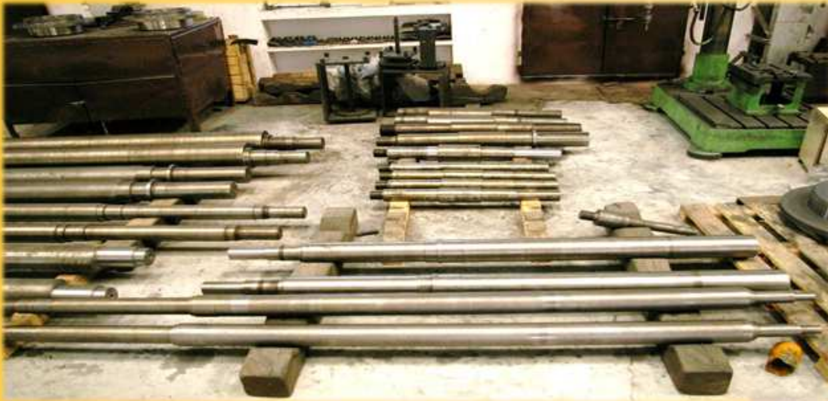
Vertical Slurry Pump Shafts ( Moc: EN8, SS316, EN19, EN24, SS304 etc)
