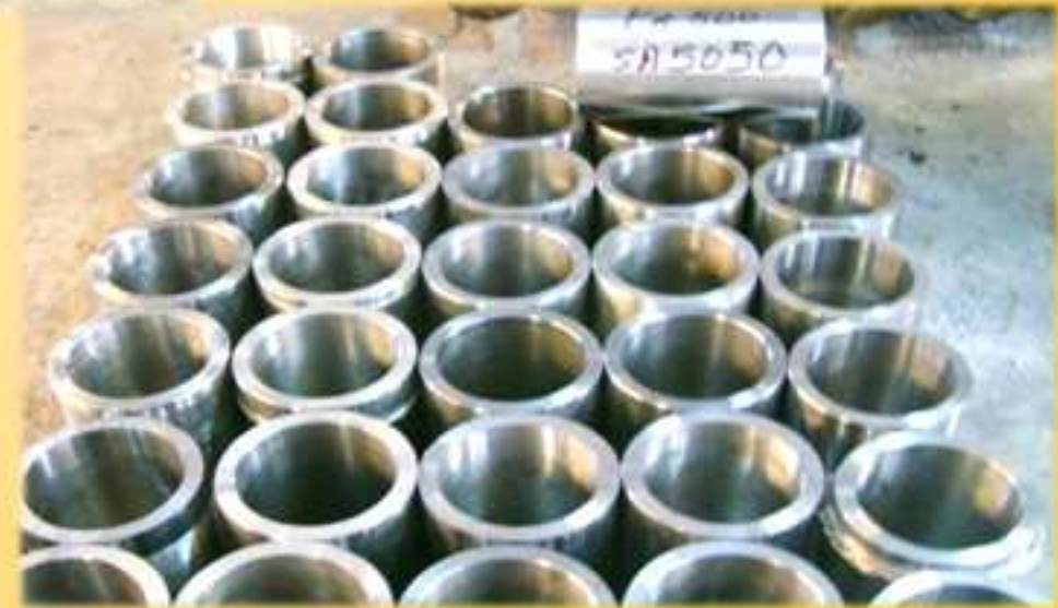
Shaft Sleeves of Heavy Duty Slurry Pump (Moc: SS316)
