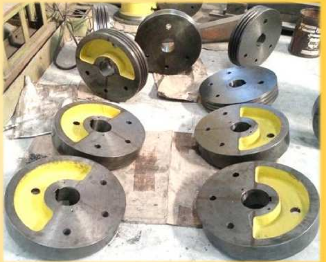
Eccentric Pulleys of Vibrating Screens (Moc: S.G. Iron)
